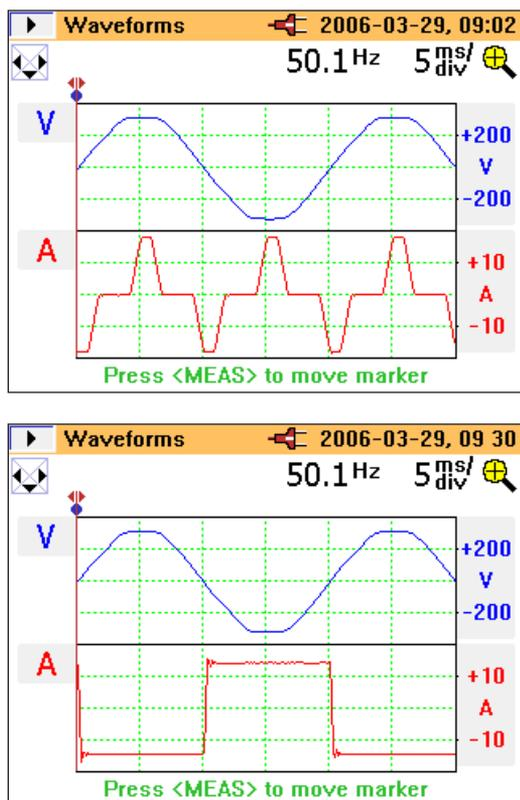
Figure 1. The dual waveform display on the Fluke 345 shows both voltage and current waveforms.
